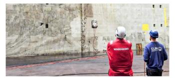
First trials with a hold cleaning robot to improve safety and quality during cleaning operations on board.
